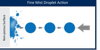
The Minncare Dry Fog 2 System produces and ultrafine droplet size that tends to bounce off of hard surfaces and thus avoid excessive condensation, corrosion and surface wetting issues associated with a fine mist bio-decontamination procedure.
